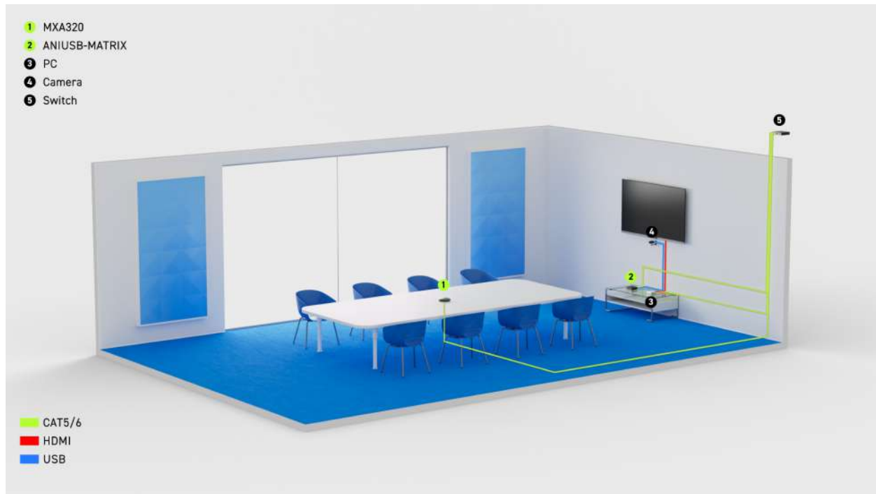
Small room equipment example
