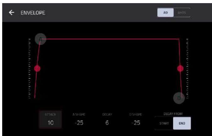
Close-up of an AD-type filter envelope.
