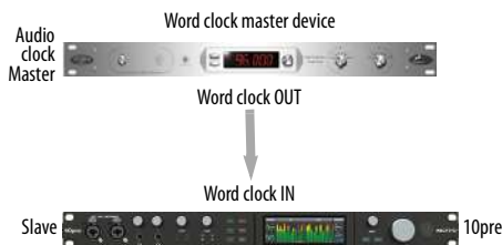
Figure 4-7: Slaving the 10pre to word clock. For the 10pre clock source, choose 'Word Clock In'.
