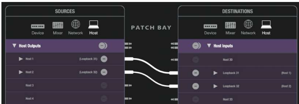
Figure 7-6: Creating loopback routing in the Patchbay. In this example, Host output channels 1-2 are being routed to Host input channels 31-32.
