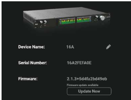
Figure 6-10: Go to the Device tab to see if there is a firmware update available.
