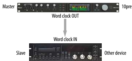
Figure 4-6: Slaving another digital audio device to the 10pre via word clock. For the 10pre clock source, choose Internal (or any source other than Word Clock , as daisy-chaining word clock is not recommended).
