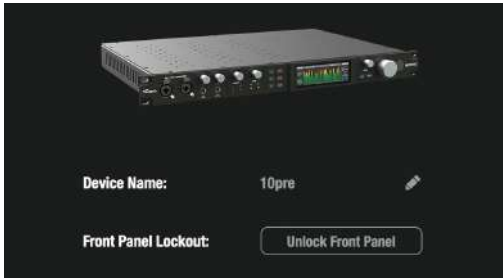
Figure 5-12: Disabling Front Panel Lockout mode in the Device tab in CueMix Pro.
