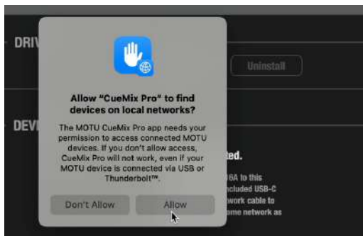
Figure 3-1: Be sure to click 'Allow' in this macOS alert, so that CueMix Pro can communicate with your 10pre device.
