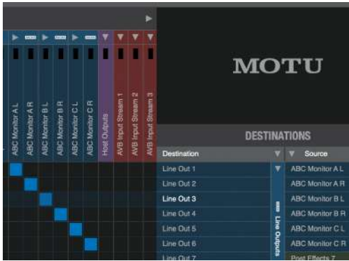
Figure 5-7: Routing the A/B/C Monitor source signals to their respective outputs. In this example, Monitor A is routed to Line Outs 1-2, Monitor B is routed to Line Outs 3-4 and Monitor C is routed to Line Outs 5-6. This is only an example; you can use any outputs you wish (analog, digital or even network channels).
