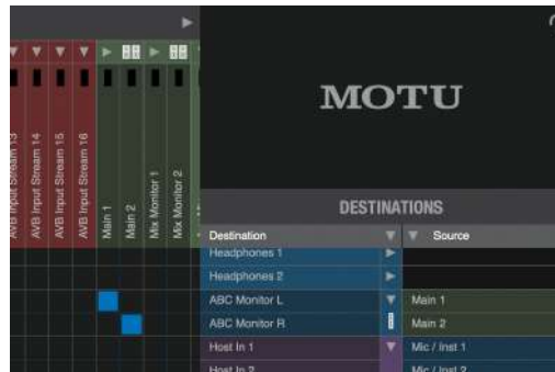
Figure 5-9: Routing host computer (DAW) output to the ABC Monitor channels (via the 10pre’s built-in mixer).
