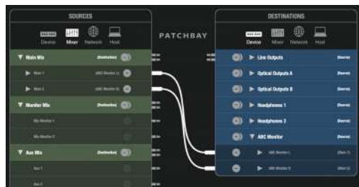
Figure 5-10: Using the Patchbay to route host computer (DAW) output to the ABC Monitor channels (via the 10pre’s built-in mixer). These are the same connections as shown in Figure 5-9.
