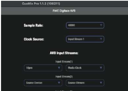
Figure 9-5: Using the 10pre's Media Clock Stream as a clock source for another AVB device.
