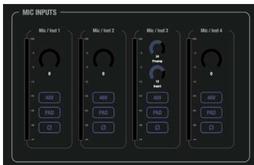
Figure 4-3: 54 dB of gain occurs before the insert point, while 20 dB occurs after. Together, they provide up to 74 dB of gain.
